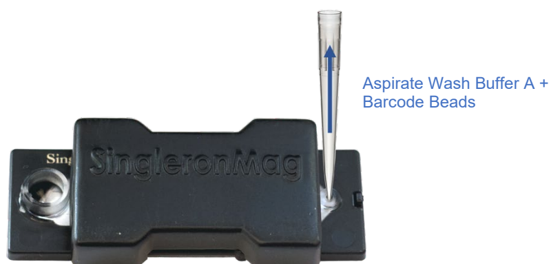
Figure 4. Collection of the Barcode Beads via inlet port
