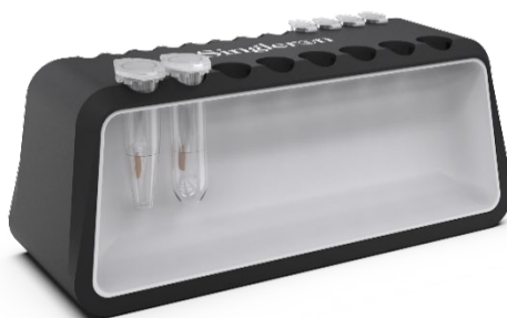
Figure 5. AMPure beads in Janus magnetic rack
