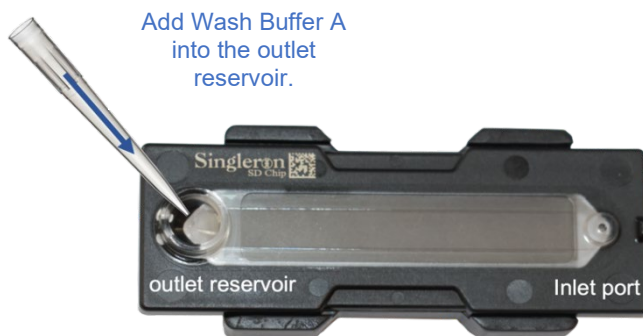
Figure 3. Addition of Wash Buffer A to the outlet reservoir
