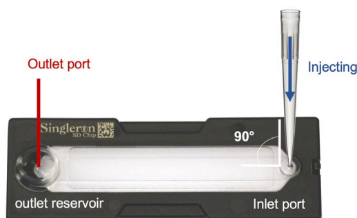
Figure 2. The position of inlet port, outlet reservoir and outlet port on the SCOPE-chip
